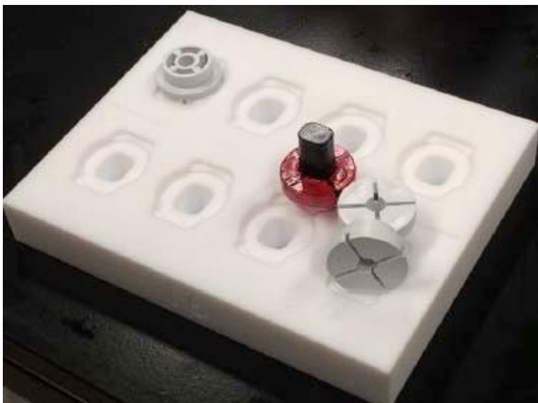
Image 3 - Larger PTFE mould with polymerised block and plastic chucks.
